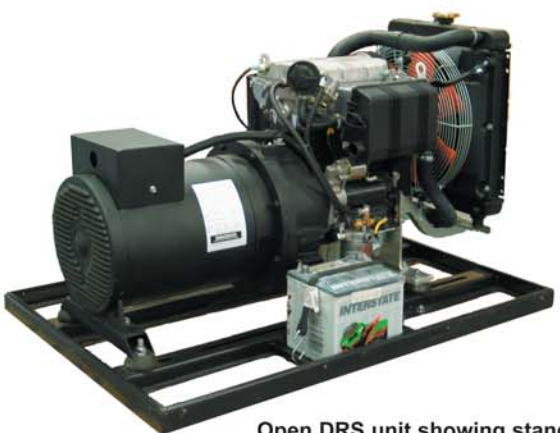
Open DRS unit showing standard features, such as: battery tray, battery, battery cables, radiator, air filter, steel skid base, and rubber isolation mounts.
